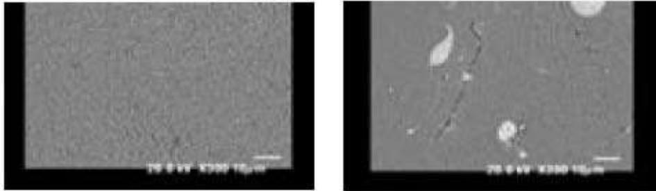
(Fig. B) Images of Good Dispersion (Left) and Poor Dispersion (Right) with TiO<sub>2</sub>
