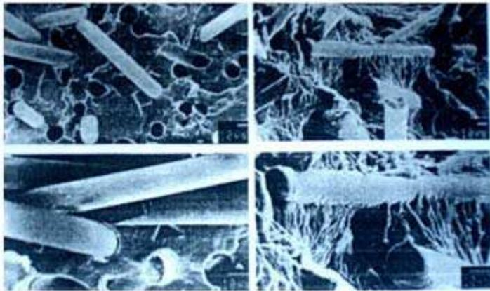
(Fig. A) SEM Images of Poor Wetting (Left) and Good Wetting (Right)
