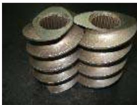
This zone pumps the homogeneous compounded melt at constant temperature and pressure. The performance of the optimally designed screws is conserved only if the excessive cooling in this zone is avoided.
