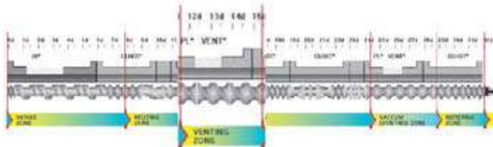
Vents are required to continuously remove air and moisture (or volatiles) during or after the melting stage. Removal of moisture to prevent hydrolysis of condensation polymers such as Nylon and PET is one of the most important requirements. Additionally, down-stream to the
