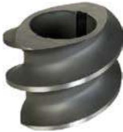
The modular design of the extruder screw assembly provides an option for a wide selection of screw elements for configuring in the 'intake zone'. The popular twin-screw elements are Single Flight Element (SFE), Schubkanten Element (SKE), Special Schubkanten Element (SSKE), Normal Right-hand Screw element (RSE), Deep flight SK element (DSK), and the newly invented Single Flight 'V' shaped (SFV) element.
